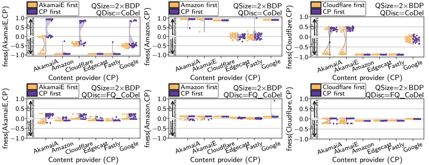
Fig. 6: AkamaiE, Amazon, and Cloudflare competing against the other content providers in the 10 Mbps, 50 ms,  $2 \times$  BDP setting using CoDel (top) and FQ\_CoDel (bottom). Amazon performs similar to Edgecast and Fastly, Cloudflare is similar to Google.
